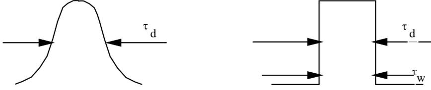
**Figure A6:** Dispersion times and pulse widths for Gaussian and square pulses The dispersion time is defined as the FWHM, the pulse width as the time containing half the pulse energy.
